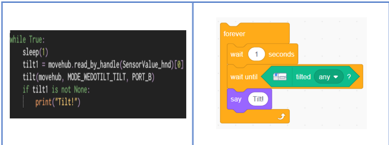
Figure 40: Tilt Sensor Activation Function : (A) Python (B) Scratch
