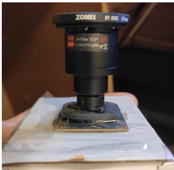
Figure 28: Interface firewire camera with IR filter
