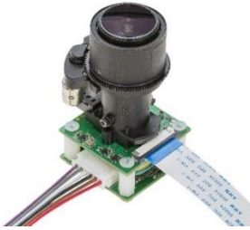
Image 35. Arducam's 8MP motorized zoom
