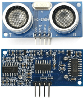
Image 27. HC-SR04 ultrasonic sensor
