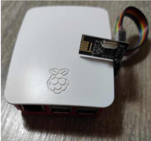
Raspberry Pi acting as Forwarder, Gateway and Broker.
