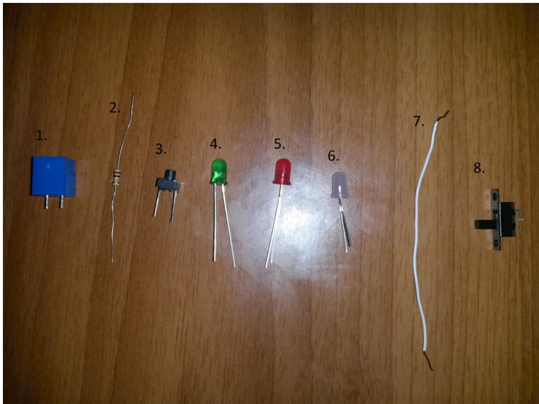
1. Clame 2. Resistance 3. Button switch 4. Green led 5. Red led 6. White led 7. Cable monoclonono 8. Switch
