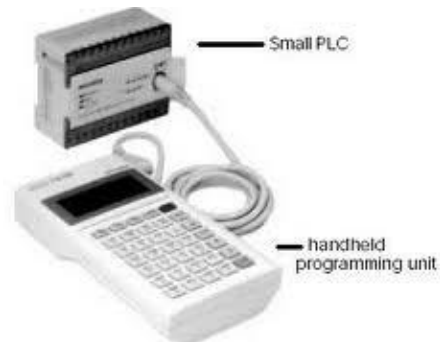
Figure Small PLC with built-in I/O and detachable; handheld programming unit.
