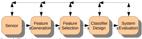
Figure 5: The development stages of a recognition system
