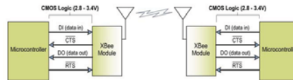
Figure 2-01. System Data Flow Diagram in a UART-interfaced environment (Low-asserted signals distinguished with horizontal line over signal name.)
