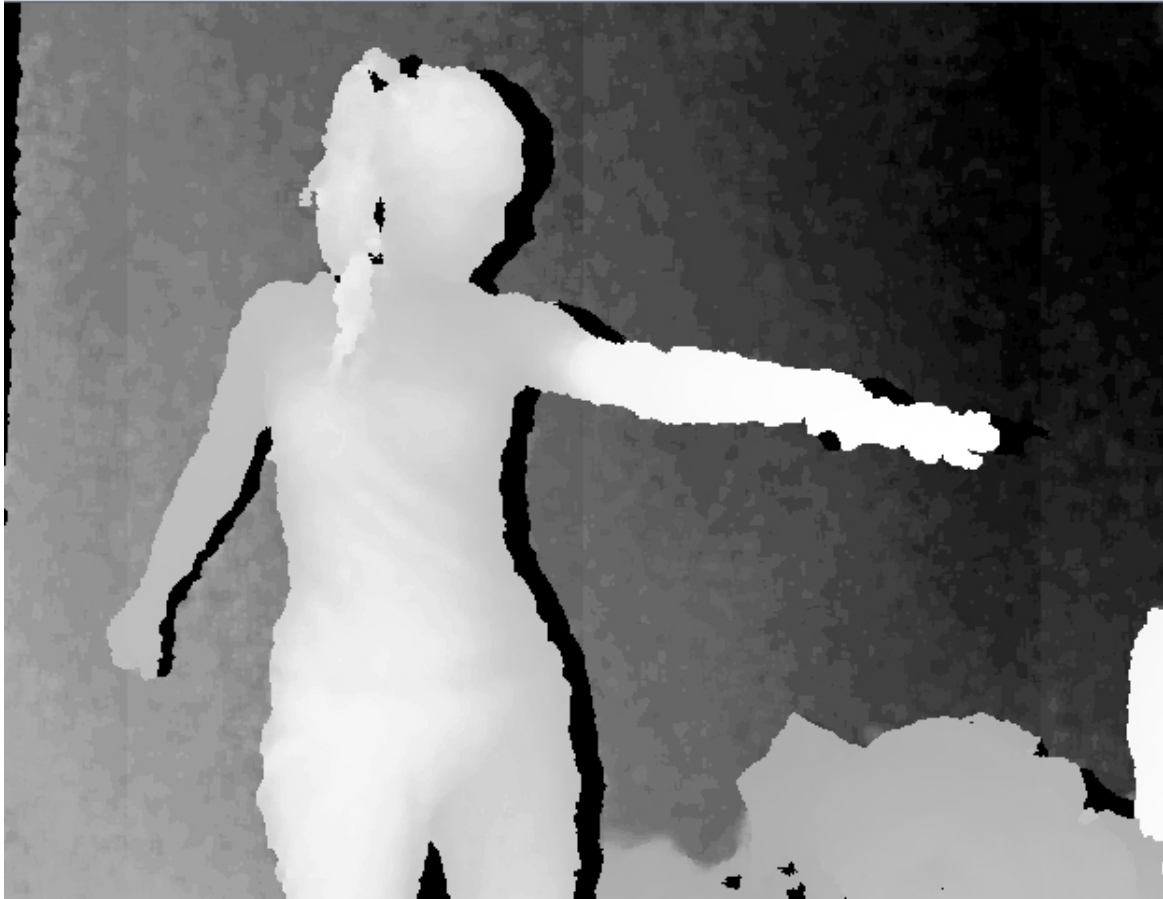
22: Grayscale Depth Mapping
