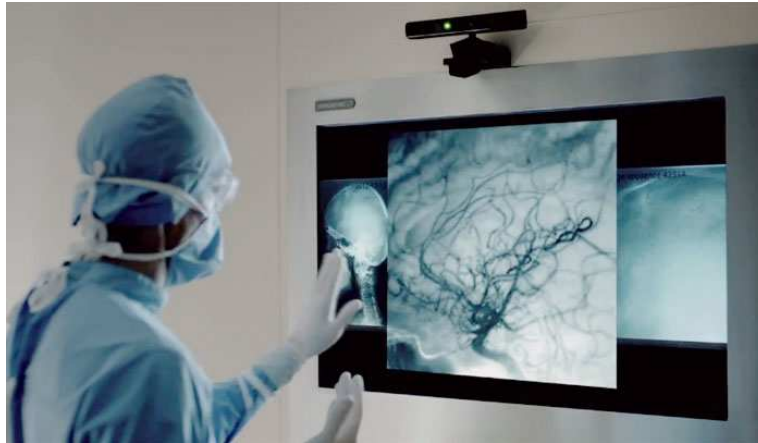
Figure 28: Controller-free interactive exploration of medical images through the Kinect.
