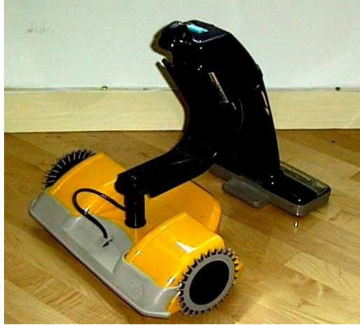
Εικόνα 3. 12-Cye, a commercially available domestic robot that can vacuum and makes deliveries at home.
