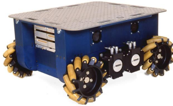
Εικόνα 3. 13 The Carnegie Mellon Uranus robot, an omnidirectional robot with four powered-swedish 45 wheels
