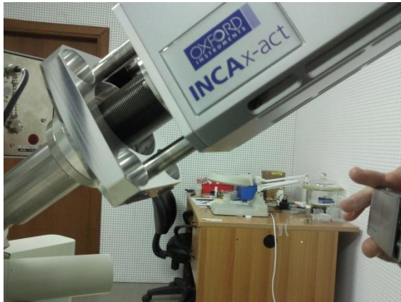
Εικ.15: Oxford Instruments INCAx-act Detector (GDD)
