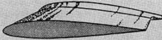
NACA 23012 wing developed at Langley Laboratory in 1934 Landing V = 100 mph
