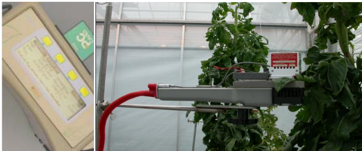
Figure 12. To the left picture of ADC LCPro+ console and to the right picture of the leaf chamber while measuring leaves of tomato plant.
