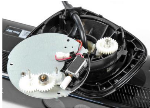
Figure 16 – Kinect’s Motorized Tilt
