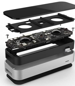
Figure 18 - The internal parts of the Leap device
