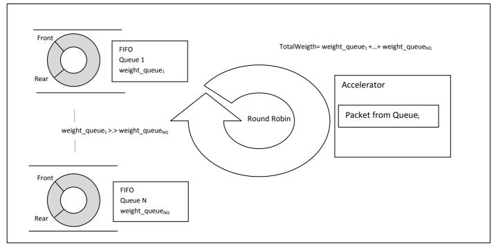
Figure 5.2-1 Schematic algorithm description
