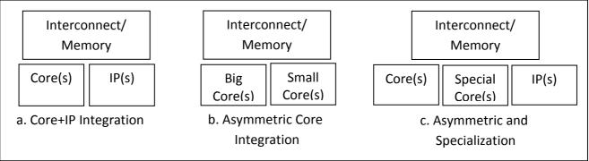
Figure 3.1-1 : Heterogeneous Architectures Under Exploration [5]
