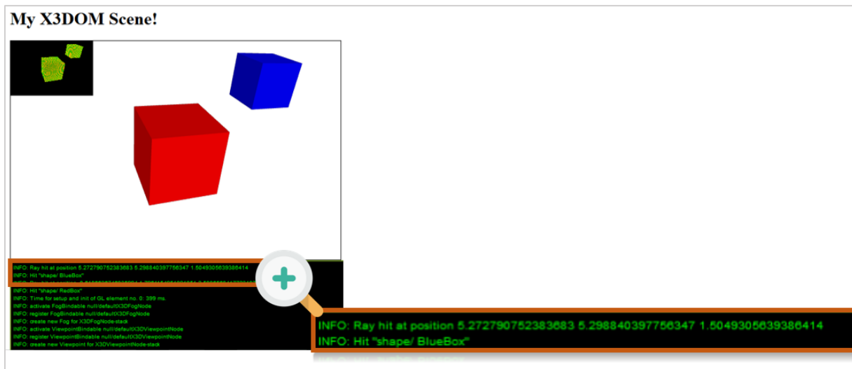
Figure 4-4. X3DOM debug mode for position coordinates
