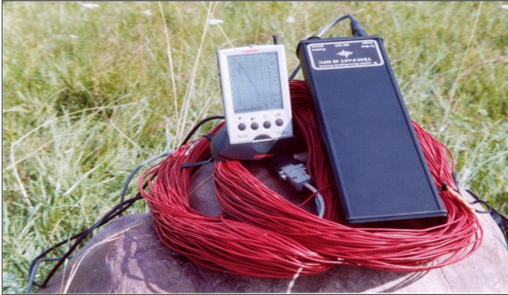
Δείγμα οργάνου TEM- FAST 48 (APPLIED ELECTROMAGNETIC RESEARCH (AEMR) TEM – FAST 48HPC, aemr.net , 2010)
