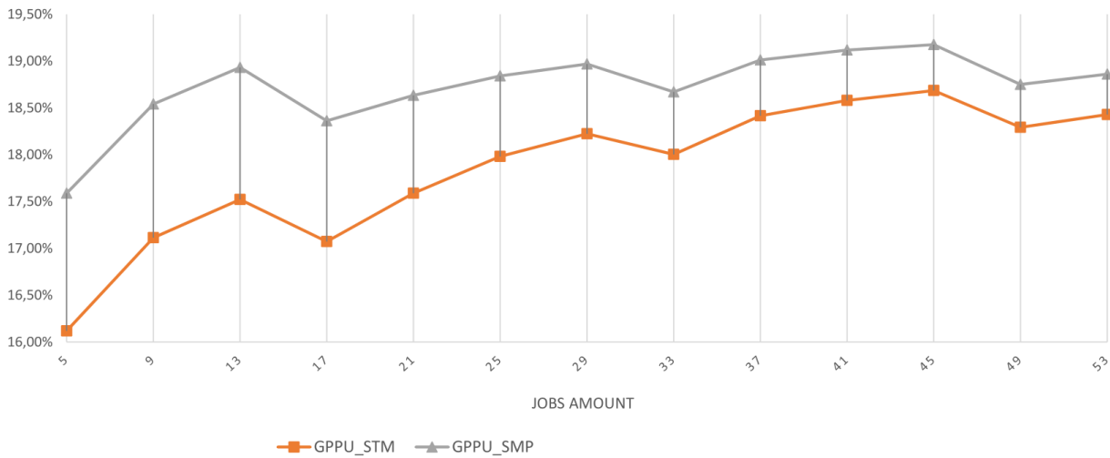
Figure 4.5: Performance gain of UHSA technology over a legacy system when offloading kernels for sobel filtering on FHD images; both memory access modes are depicted.
