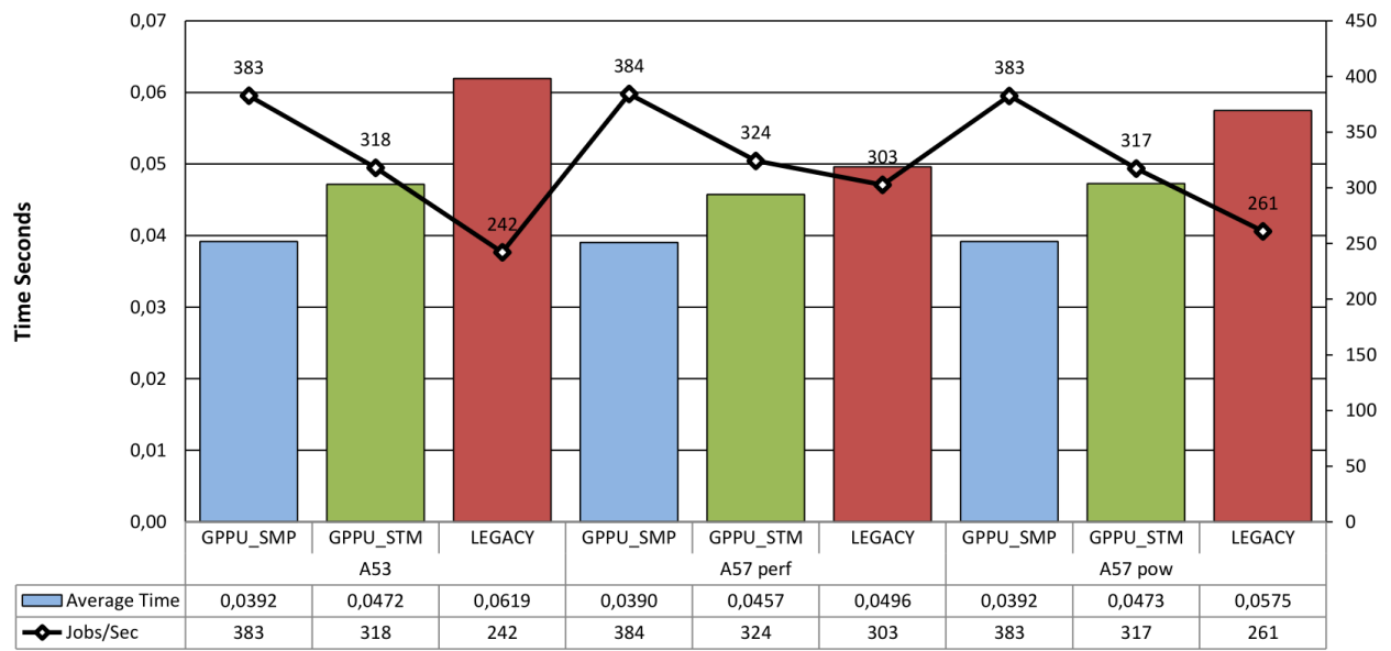
Figure 4.6: Latency and jobs per second; Matrix multiplication 15 kernels offloaded to hardware accelerator, utilizing every described mode.
