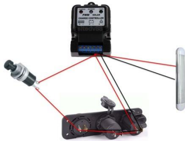
Attaching the Power Socket and LED to the Regulator
