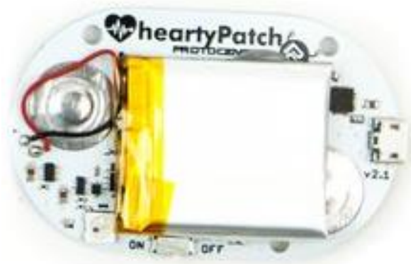
Figure 2.1.2: The HeartyPatch with a battery attached. [2]
