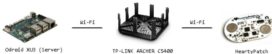
Figure 3.3.2: Network topology for the HeartyPatch.
