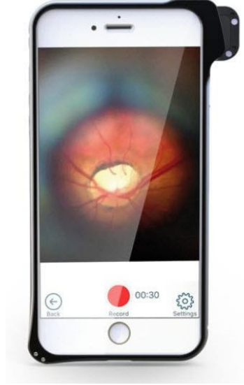
Figure 1.1: A special fundus camera attached on a mobile phone Image taken from https://www.d-eyecare.com/en_US/howtouse#assembly
