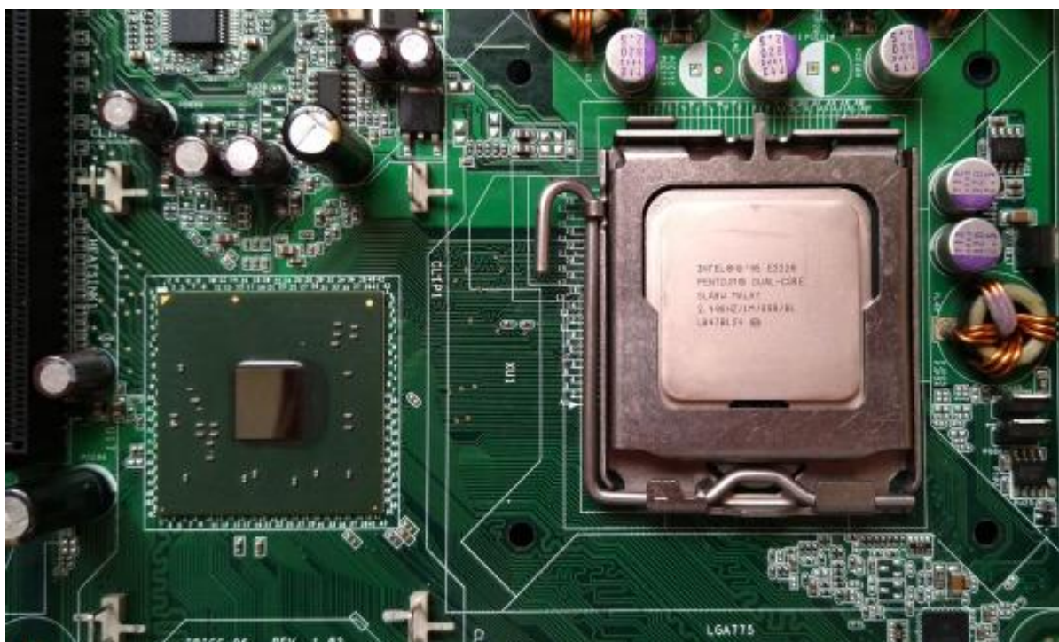
Figure 10: Complete chipset (LGA775 specifically) on a circuit board (Motherboard) with the Chip fitted (Intel Pentium E2220) and its Northbridge (Small black square on the left) [F.11]
