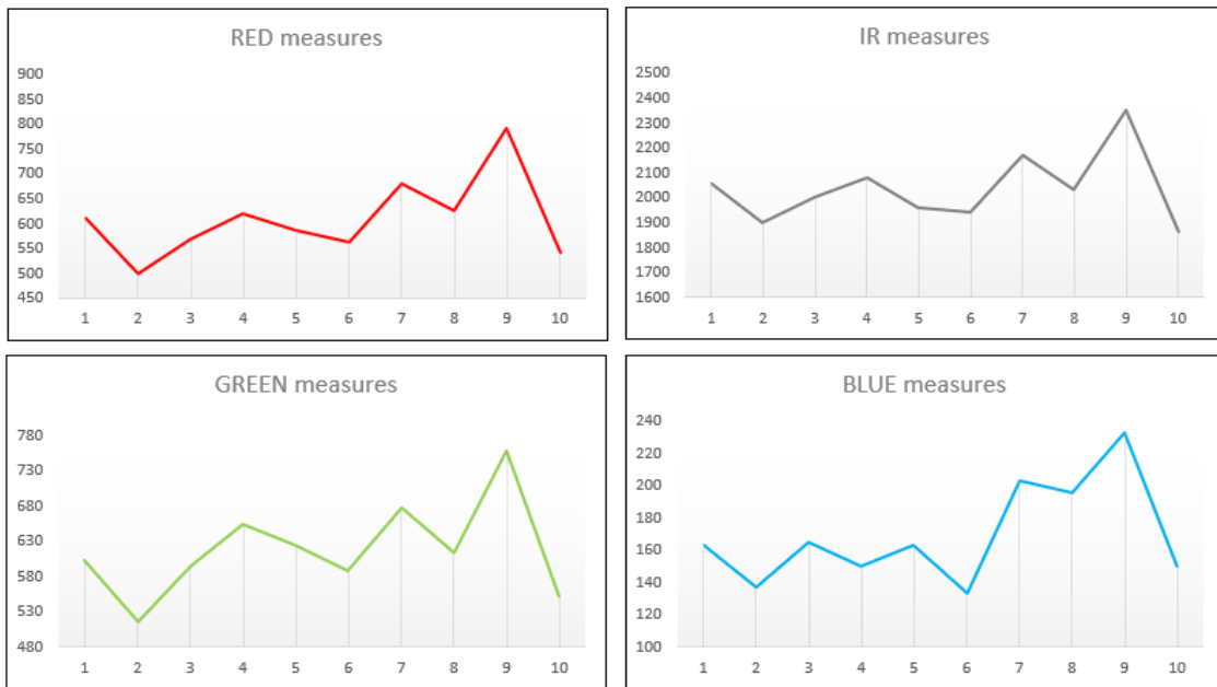
Fig. 59 LEDs measure curves for lemon leaves.
