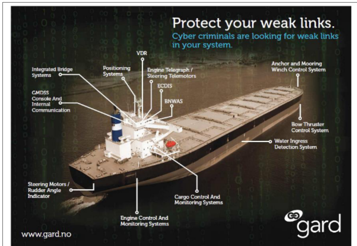
FIGURE C.1: Cyber Security weak point in a vessel, by gard.no.
