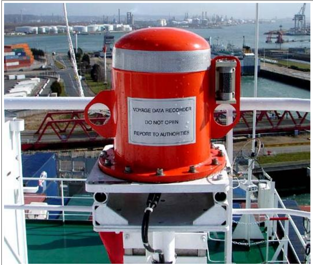
FIGURE 3.9: A Voyage Data Recorder (VDR), the "black box" of a ship, on the container ship SMA CGM Nabucco by wikipedia.org.
