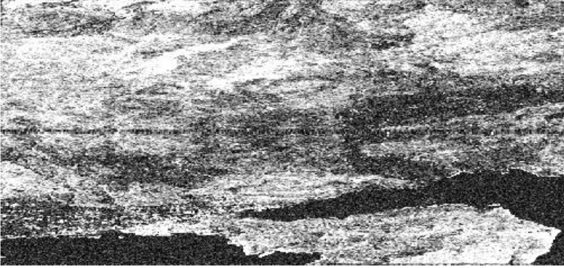
Figure 14. Coherence map of part of Western Crete (interferogram for October 2017 and December 2017).
