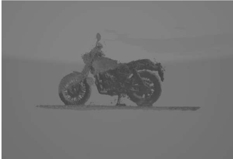
Figure 52 Custom 360 scene, lighting conditions setting 2, mesh produced using Marching Cubes algorithms
