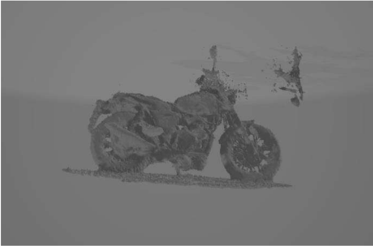
Figure 49 Custom 360 scene, lighting conditions comparison, mesh produced using Marching Cubes algorithm
