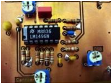
Photo 2. The modulator is based on the well known MC1496 IC, which is able to suppress the carrier for more than 60dbs
