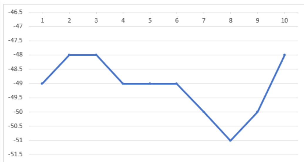
Figure 20 - Results for RSSI at 1m with wide brick wall
