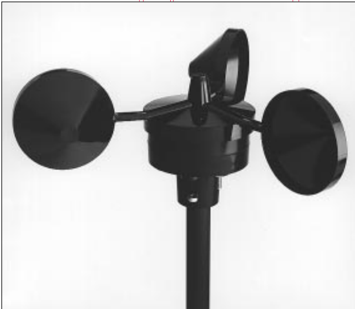
The Maximum #40 has three conical cups molded in one continuous piece. Cup rotation induces a sine wave voltage in a single coil by a four pole magnet. Two sine wave cycles are produced for each revolution of the cups with the frequency directly proportional to windspeed.
