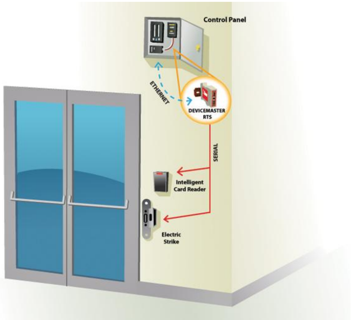
Access control system
