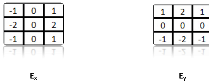
Figure 2.4 – Sobel operator (two 3x3 masks): Mask E_x detects vertical edges while mask E_y detects horizontal edges
