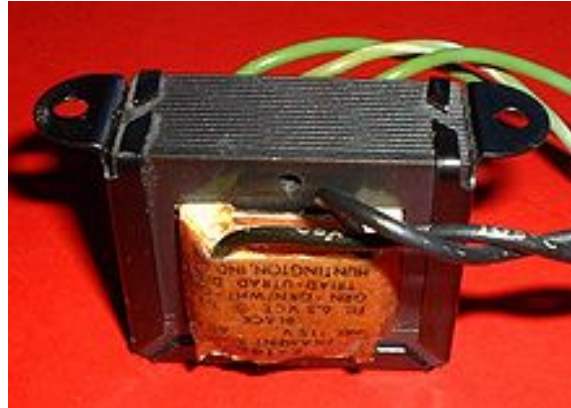
Image 2.1 Laminated core transformer showing edge of laminations at top of unit.
