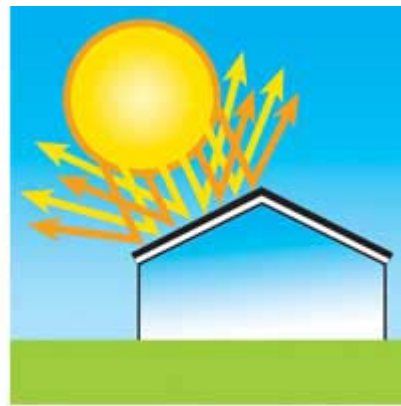
FIG. B ROOF WITH COOL ROOF PAINT
