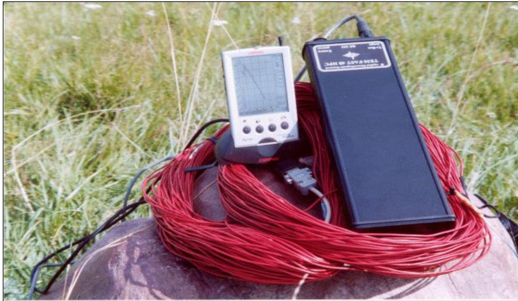
ΕΙΚ 11: Δείγμα οργάνου TEM- FAST 48 (APPLIED ELECTROMAGNETIC RESEARCH (AEMR) TEM -FAST 48HPC, aemr.net, 2010)
