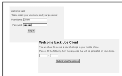
Figure 8: Screen sequence where the user logs in to the web service and gets forwarded to a page that requests the second authentication factor
