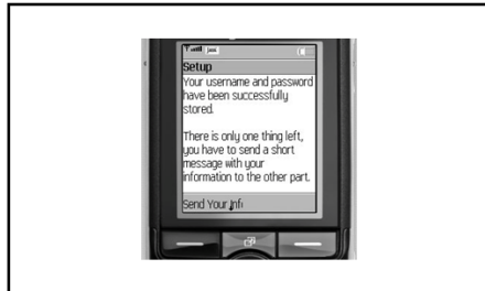
Figure 7: Screenshot from the user's mobile phone where he sends his activation data to the server's side
