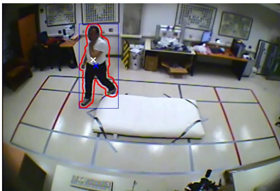
Figure 10: The Kalman filter as shown in our method. The blue “x” is the computed center of mass (centroid of contours), whereas the white “x” is the estimated center of mass by the Kalman filter
