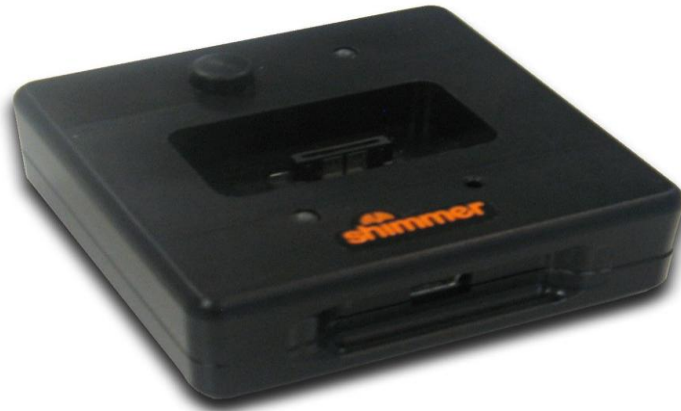
Εικόνα 7: USB Reader: Dock for programming and charging the Shimmer
