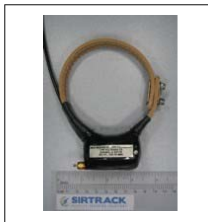
Proximity logger built for raccoons
