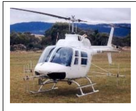
Helicopter kitted with Sirtrack three element fixed Yagi antennas
