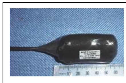
High power rhino horn implant
