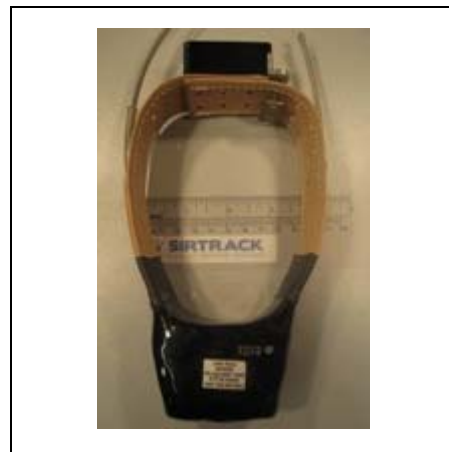
PTT/VHF collar with Sirtrack's time release
