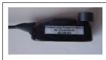
Trap transmitter with removeable magnet to activate the transmitter.
