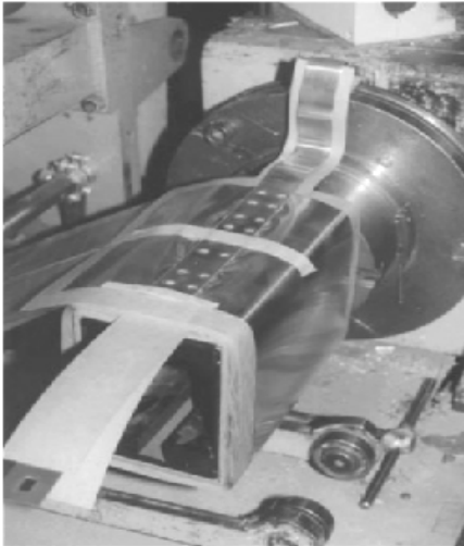
Spiral Sheet Low-voltage Winding
