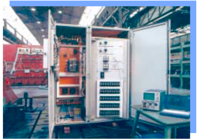
GSE type AVR under Test
