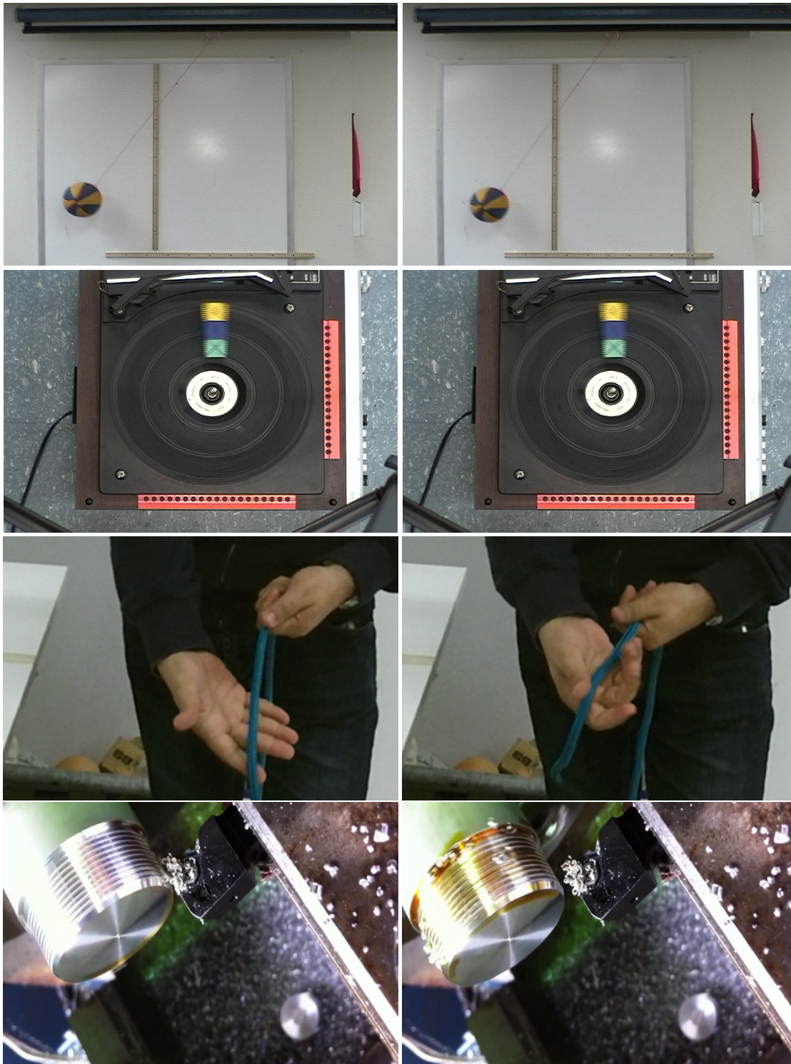
FIGURE 4.5: Indicative results from experiments in four videos (pendulum, turntable, rope, machine). A pair of frames is selected from each video, a random one (left) and one at a temporal distance equal to the period length computed by the proposed method (right).
