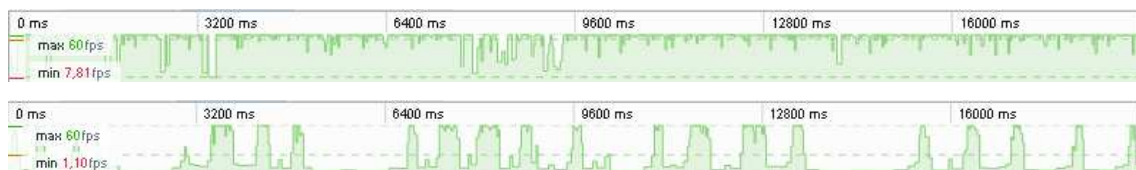
Figure 5.4 Comparison of frame rate during simple streaming (above) and during sketching (below). Negative spikes denote that the user is sketching on the canvas.
