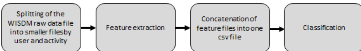
Figure 4.2: The data handling, processing and analysis pipeline in WISDM
