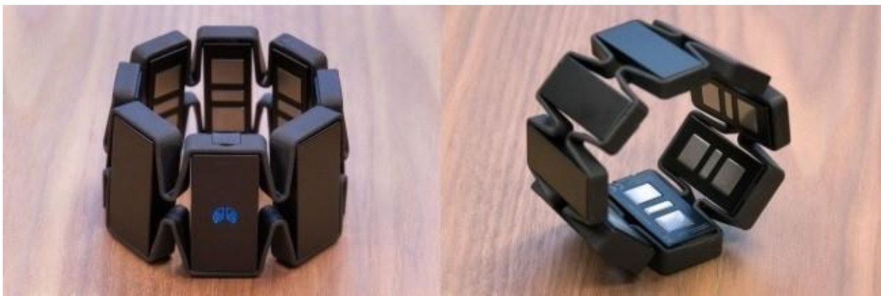
Figure 13: MYO a muscle tracking sensor device [32]
