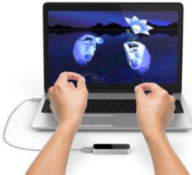
Figure 10: User's interaction with the computer through the finger motion tracking that Leap offers [26]
