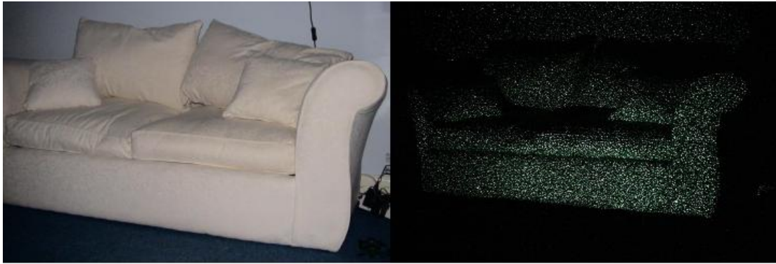
Figure 1.4: RGB image of a sofa (Left), The same image as the Kinect sensor sees it (Right).
