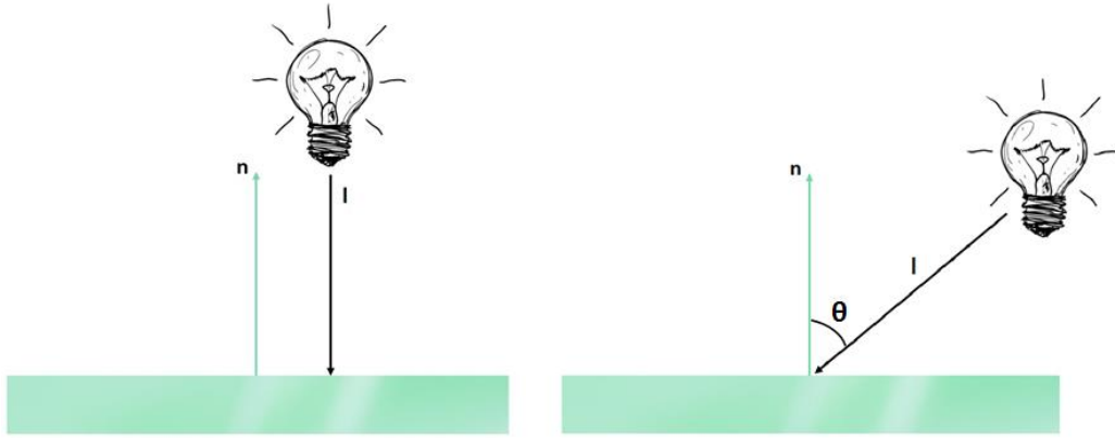
Figure 2.9: Illumination of a diffuse surface when the light direction is vertical to the surface (right) and when there is an angle between them (left).
