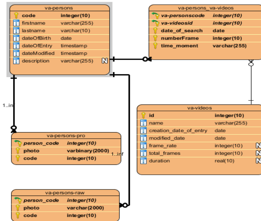
Figure 31 Entity and Relationship Model of the database
