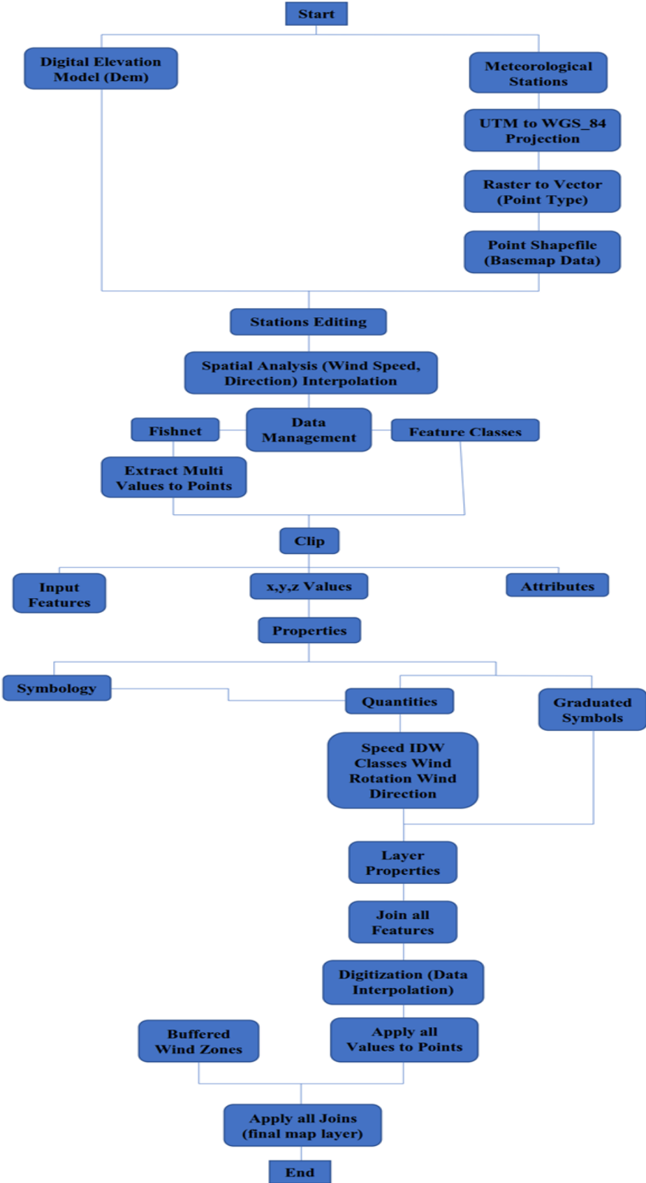
Chart 4: Flowchart for calculating wind potential, especially applied for this study.
