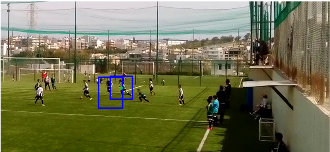
Figure 5.3: The KCF tracker does not recover from full occlusion
