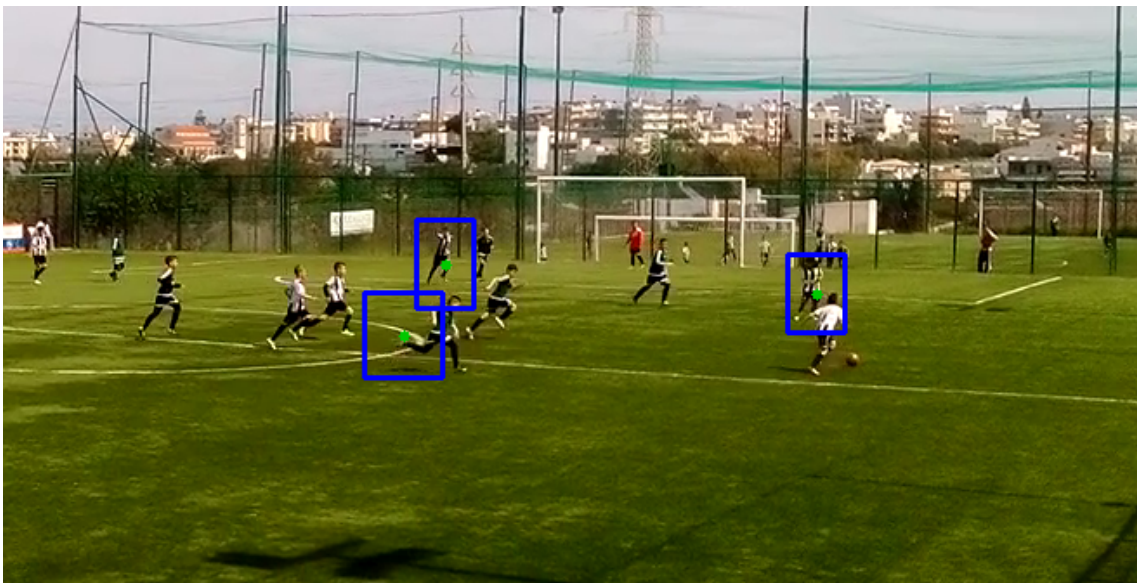
Figure 5.5: MIL fails under full occlusion
