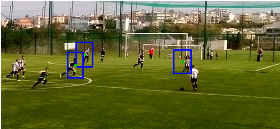
Figure 5.4: When the full occlusion is about to happen
