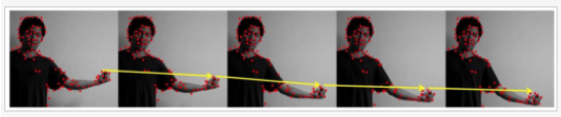
Figure 2.1: Example of fist tracking using one Lucas-Kanade-Tomasi(LKT) tracker [5]
