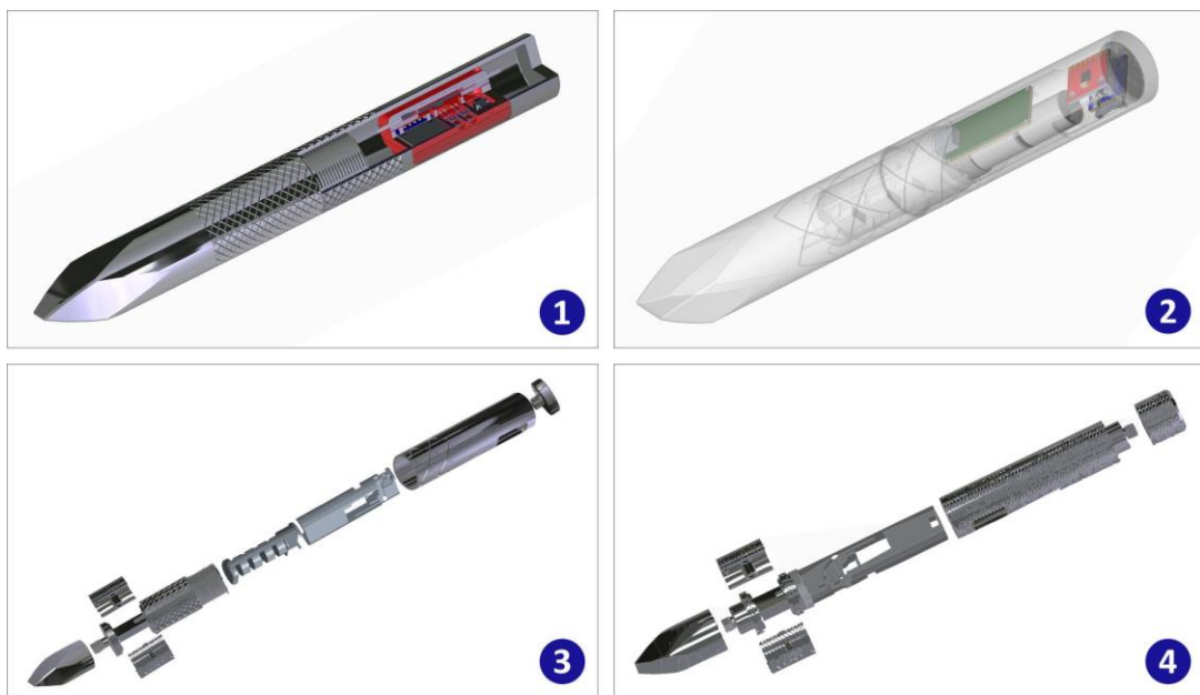
Figure 1: The design stages of the smart tool for percussion carving, from the initial design (1) until the optimized version (4), including the two intermediate builds (2) and (3).
