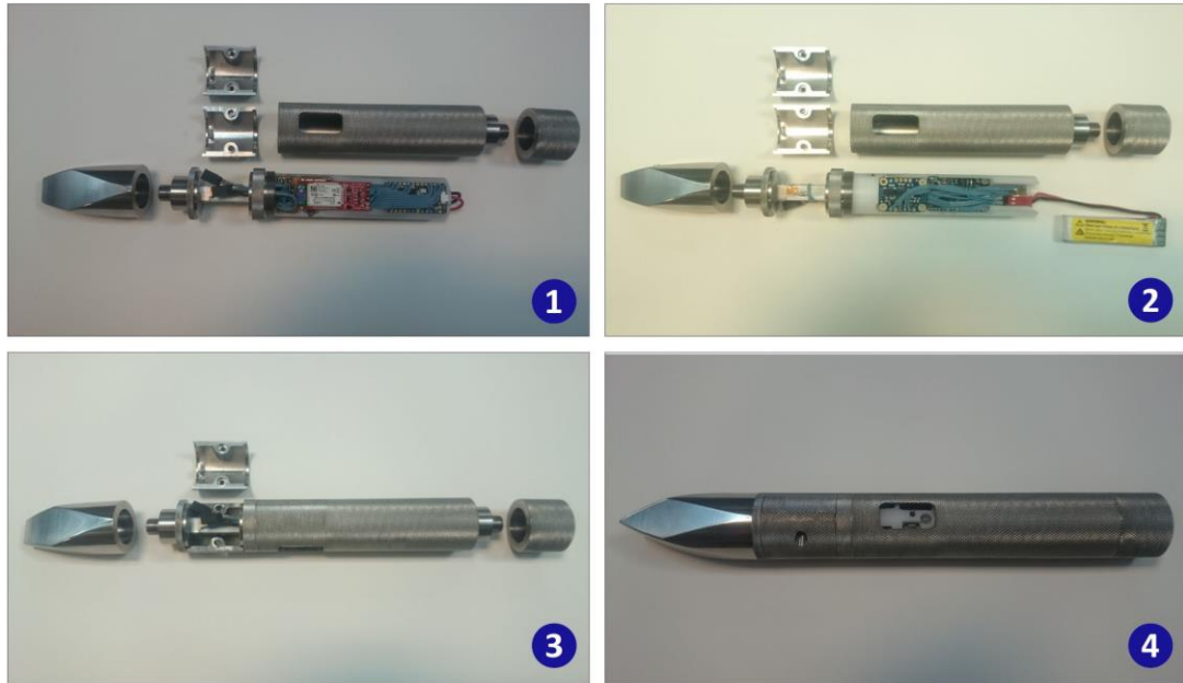
Figure 2: The optimized smart tool for percussion carving prototype in various assembly steps. From the step of the fully expanded form, illustrating the front face with the Bluetooth unit and the central processing unit (1), while the back face illustrates the inertial measurement unit, the central power unit and the battery (2), which has been installed into the electronics module. Also, presented the fully assembled smart tool (4) and the sum expanded form of intermediate step (3).
